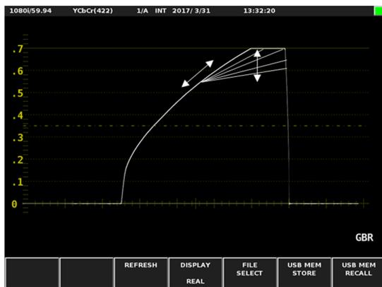
Adjustment of Knee Point and Slope (HDR)
